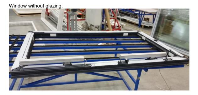
!!! Note: Remeber positions of glazing supports shown below. They must be insterted again in the same places during reinstallation of the glazing.
